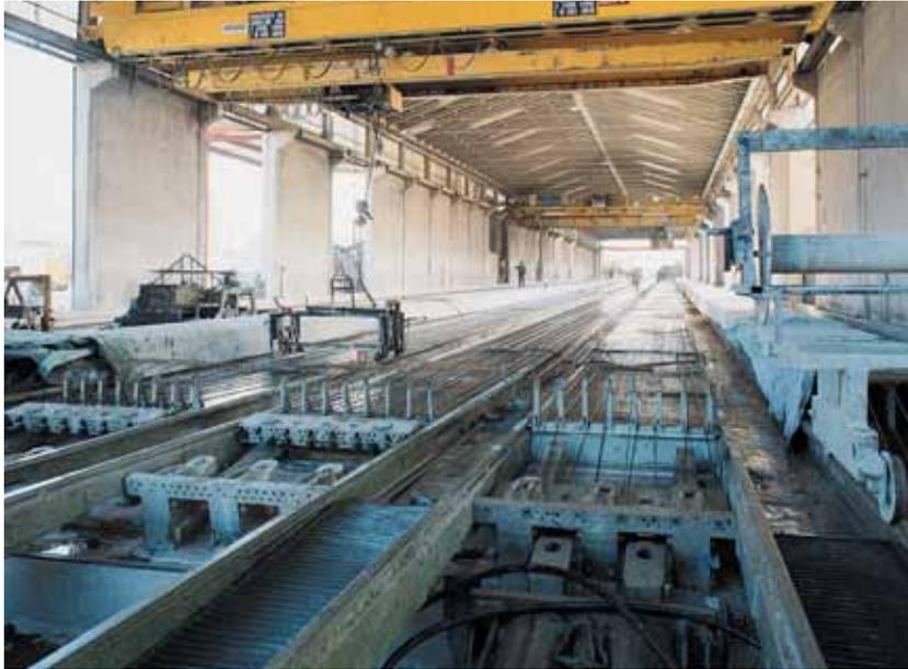
*Fig. 2.3 Prestressing reinforcement stretched on the casting bed*
