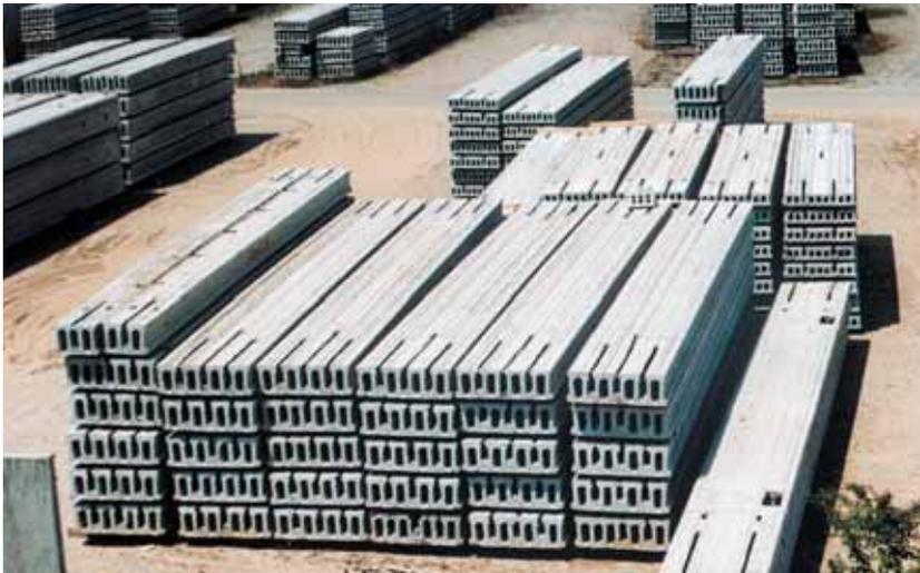
*Fig. 2.6 Hollow core slab storage yard*
