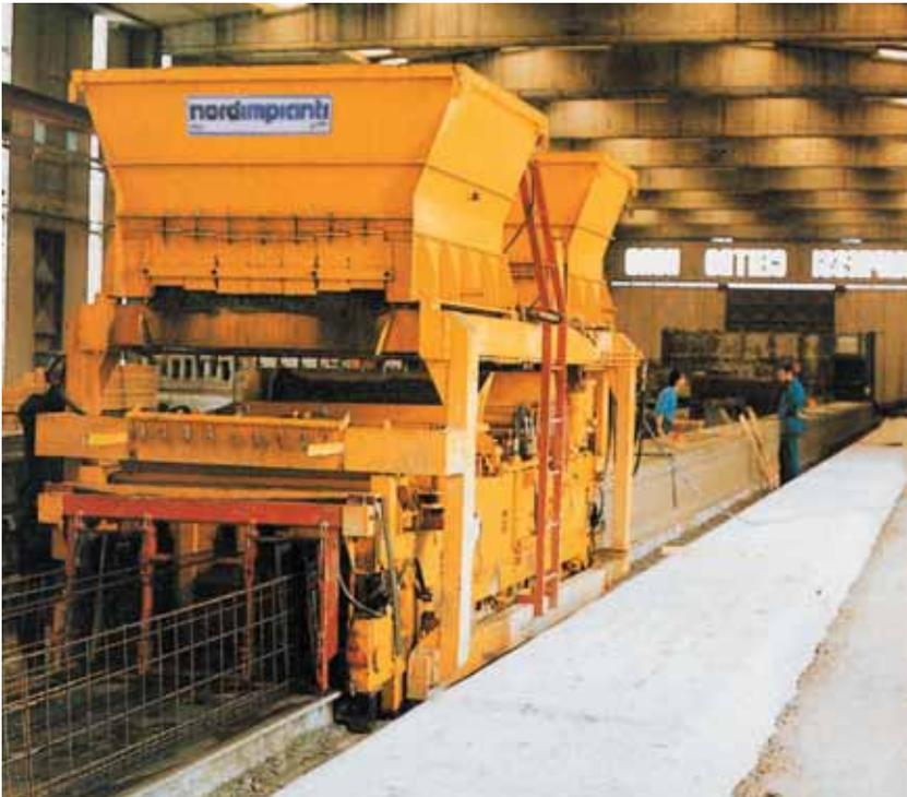
Fig. 2.1 Slide-mould machine (slipform procedure)
