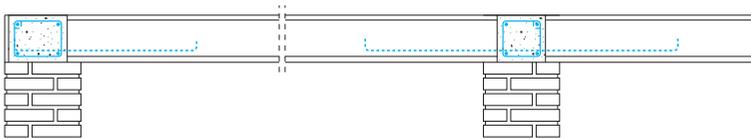
Fig. 4.6 *A simply supported hollow core floor*
