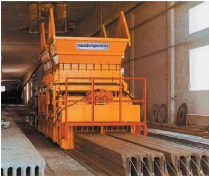
*Fig. 2.4 Continuous casting of concrete*
