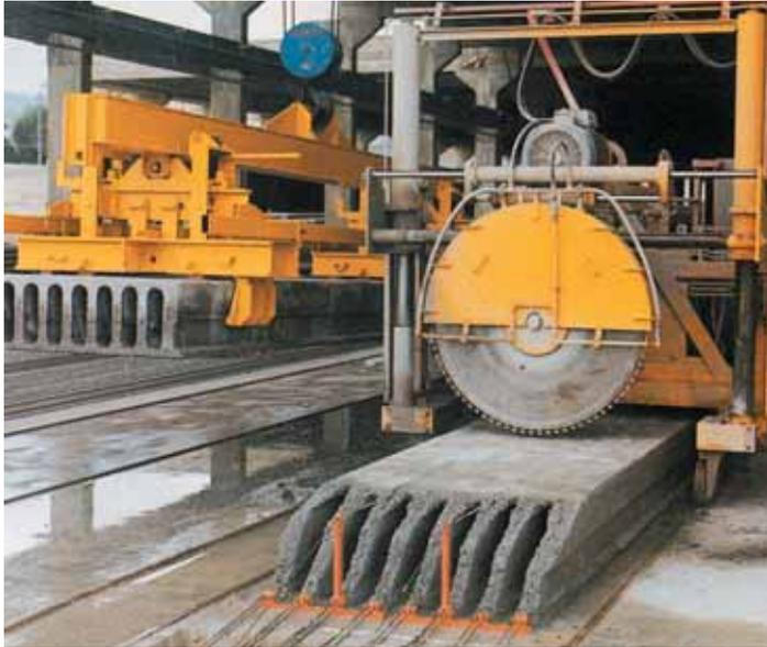
*Fig. 2.5 Cutting of slabs and their removal from casting bed*
